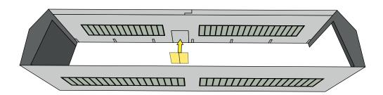
7. Detach the Inner Roof. Then locate the tabs and pre-fold them along the score lines.
