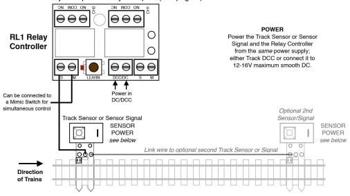
Using one Track Sensor or Sensor Signal the relay will close as soon as the train passes it and then open again about 7 seconds after the last part of the train has passed the sensor. However if you use a second Track Sensor/Signal and link it to the first as shown above, then the relay will close as the train passes the first sensor but not open until the train passes the second sensor, so in this way you can make something operate while a train is located in a particular section of track.
