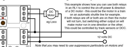
solenoids to prevent interference (these are usually fitted to loco motors)
