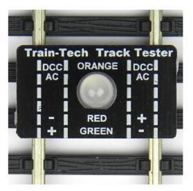
The Track Tester works on OO, HO, TT or N gauge track and enables you to quickly test for DCC or DC power and also help locate faults at track joints and points etc.
